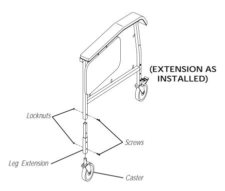
FIGURE 1 - INSTALLING 5-INCH LEG EXTENSION KIT - MODEL 6908A
